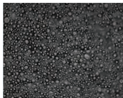
FIGURE 11—Convocal microscopy of a matte, soft-feel PUD (100x mag/size 178x134 µm).
