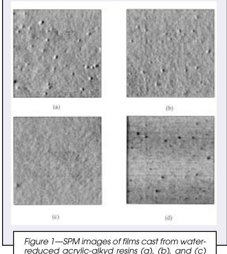
Figure 1—SPM images of films cast from waterreduced acrylic-alkyd resins (a), (b), and (c) are deflection images of C6, C7, and C8, respectively. (d) is a friction image of C7.
