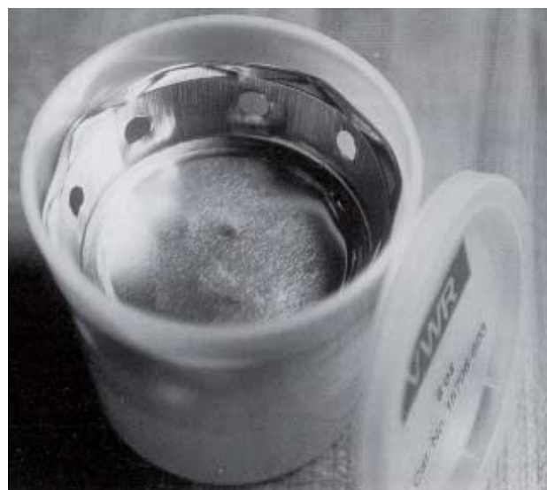
Figure 6—Photo of open sorption cell with aluminum pan.
