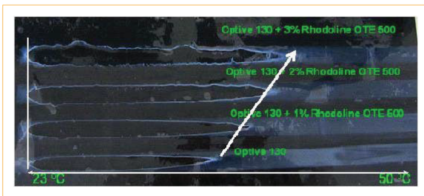
Figure 8 —Redispersion and coalescing process of latex particles with and without Additive 1.
