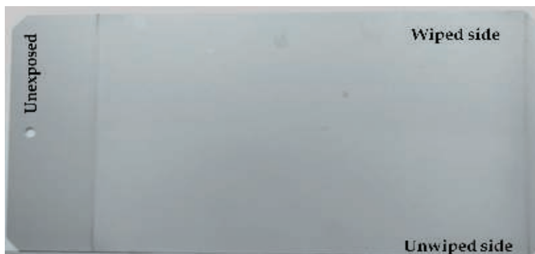
FIGURE 11—LE AMSS 36375 coating after two years of weathering exposure at Monegeetta, showing only slight change on the exposed area when compared with the unexposed portion.
