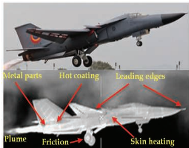
FIGURE 3—An F-111 aircraft viewed visually (top) 19 and through a Band III TIR camera (bottom). TIR image provided by DST Group.
