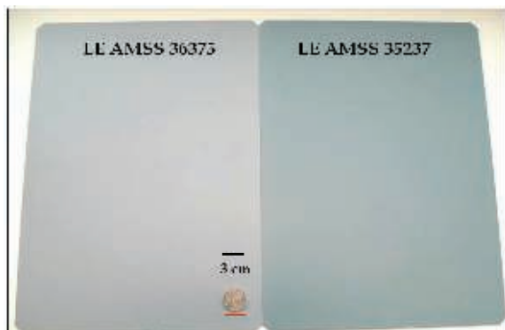
FIGURE 9—Spray-applied LE AMSS 36375 (left panel) and LE AMSS 35237 (right panel) under D65 illuminant conditions (panel sizes 0.3 x 0.4 m).
