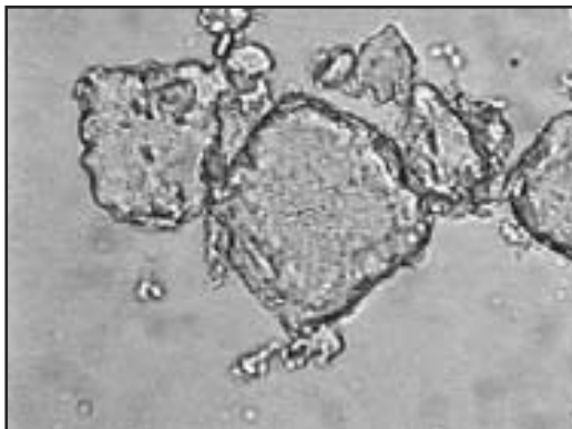
Figure 2—Photomicrograph of the latex from Figure 1 containing a small amount of HEUR thickener. Because there is not enough HEUR to cover at least 50% of the surface, bridging flocculation occurs. These flocs are large and very difficult to shear apart.
