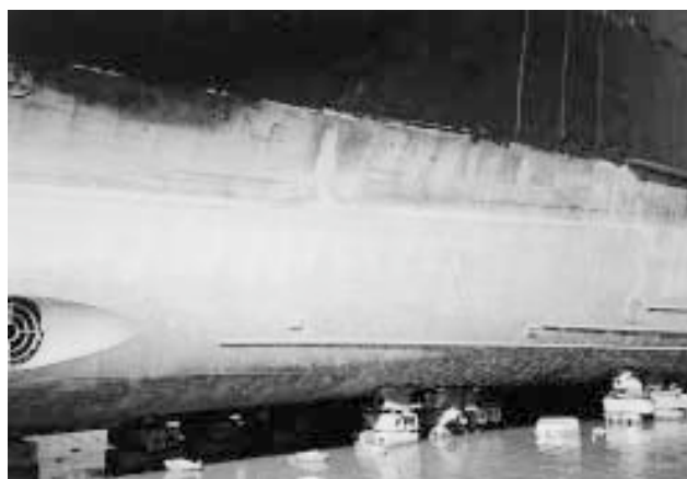
Figure 7—Pictures obtained from the ship test for the Fong Seong No. 727 ship, which had sailed 26 months in the sea around Guam.
