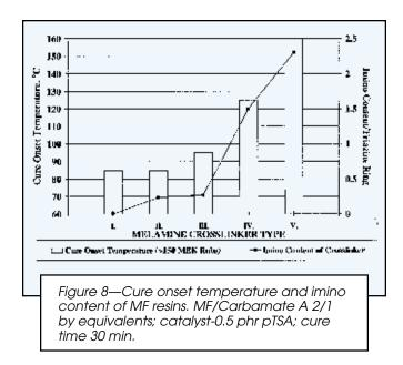
imino content but shows a marginally higher onset temperature than the HMMM types (95°C vs. 85°C). This difference is probably due to the higher boiling point of the butyl alcohol displaced during cure.
