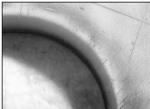
Figure 10—An example of picture framing or fat edge in a coating for agricultural implements. Original photograph at 20X.
