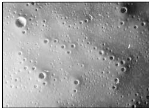
Figure 18—Pinhole gassing: acrylic electrocoat over galvanized steel. The rupture voltage had been exceeded and there was excessive gassing. Original photograph at 15X.
