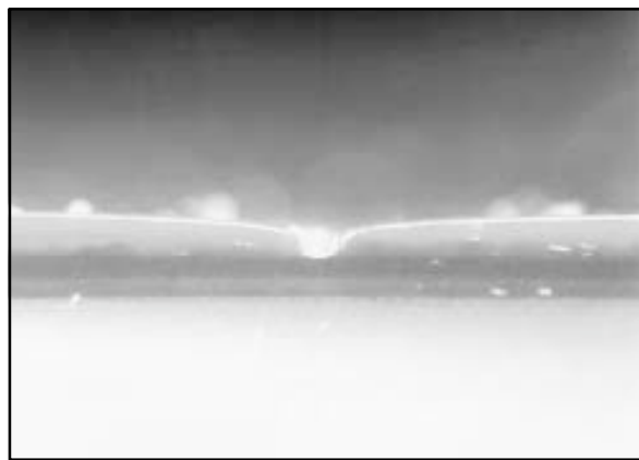
Figure 19—Cross section of a blowout pop which originated in the basecoat or clearcoat. Photograph taken at 152X.
