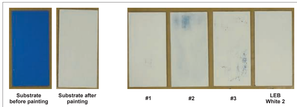
FIGURE 5— Panels with White Bases before and after shower test.
