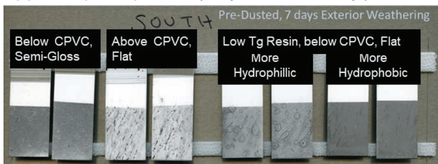
FIGURE 16 —Scanned image of outdoor shedding results after seven days of exposure from pre-dusted paint chips provided in duplicate. Samples were initially homogeneous and dusted to similar grayscale values.
