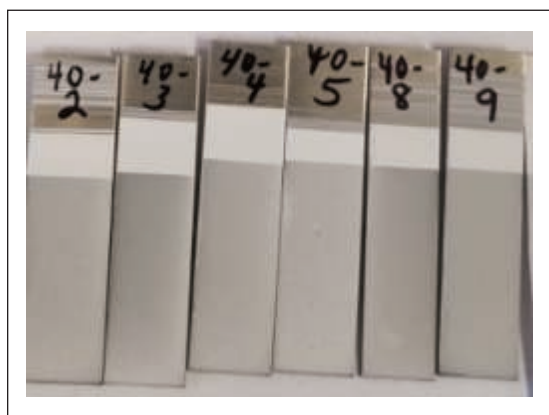
FIGURE 7—Optical image of typical dustings for a selection of paints used in this study.
