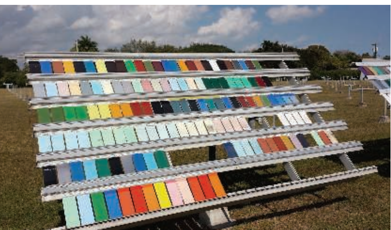
Figure 4 —Arkema test fence (photo taken January 2015) showing Florida weathering series for 70% PVDF-acrylic hybrid waterborne coatings (air-dry or low temperature bake). Many of the panels on this fence have already been on exposure for over 10 years, while showing excellent color retention.
