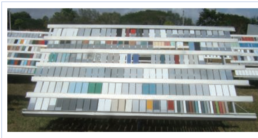
Figure 6 —Commercial baked finishes, many of them 70% PVDF coatings with mica and metallic flake pigments. The panels on this fence have been on exposure in south Florida for 10–20 years.
