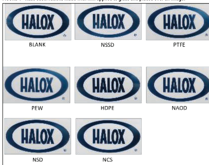
FIGURE 4—Haze observations made with film applied to glass and placed over an image.
