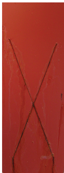
FIGURE 1—336 hour salt fog exposure.
