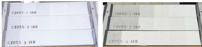
FIGURE 4—Semi-gloss benchmark series: initial and seven-month Los Angeles exposure.
