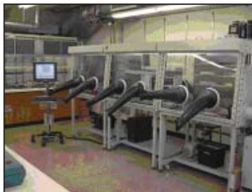
Figure 2—Triple glovebox housing the synthesis system.
