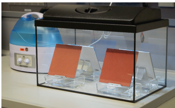
Figure 4: Modified aquarium with a cold water vapour condenser attached to it to study leaching
