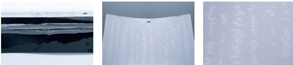
Figure 3: Images of Binder 2, showing film-forming residue in the pocket, shiny snail trails per microscope, and shiny still trails on the foil surface.
