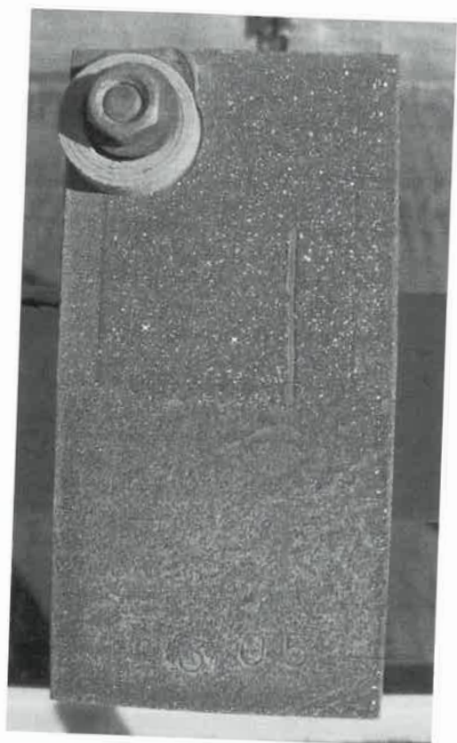
Figure 5—Photograph of the sample corresponding to system 4 (chlorinated rubber pigmented with micaceous iron oxide (supplier 2) applied on hot-dip galvanized steel weathered in the humidity condensation cabinet and cleaned by wire brushing, after 11 years of exposure in the Madrid atmosphere. Small zones without coating on the lower half of the specimen, where only one coat was applied, are observed.
